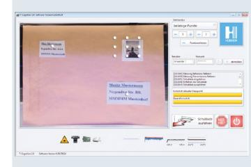
The generated image is shown on the user interface and the area to be examined is set using individual points and/or grid points.
