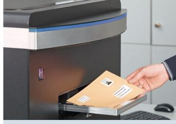
The postal deliveries that are to be checked are placed on the retractable tray and are photographed while drawing in.
